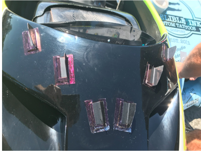
EXAMPLE OF NON-CONFORMING STRAKES
