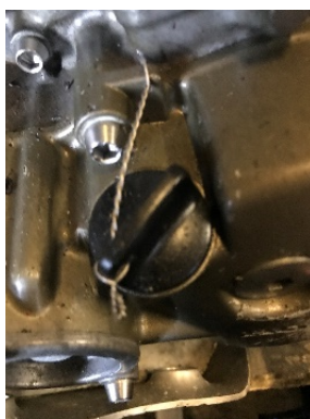
OIL FILLERS TO BE WIRED CORRECTLY SO THEY CANNOT UNDO
