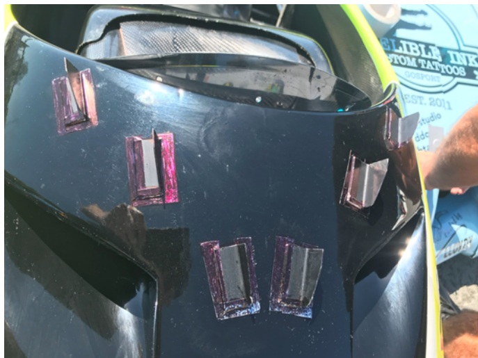
EXAMPLE OF NON-CONFORMING STRAKES
